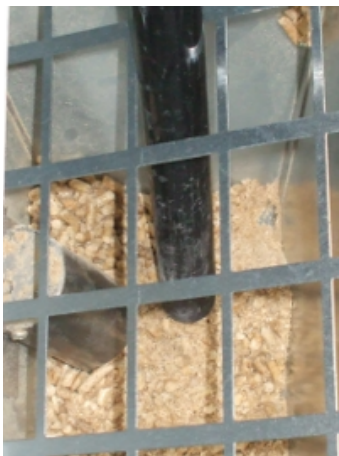
Fig. 39 - Hopper and auger cleaning
