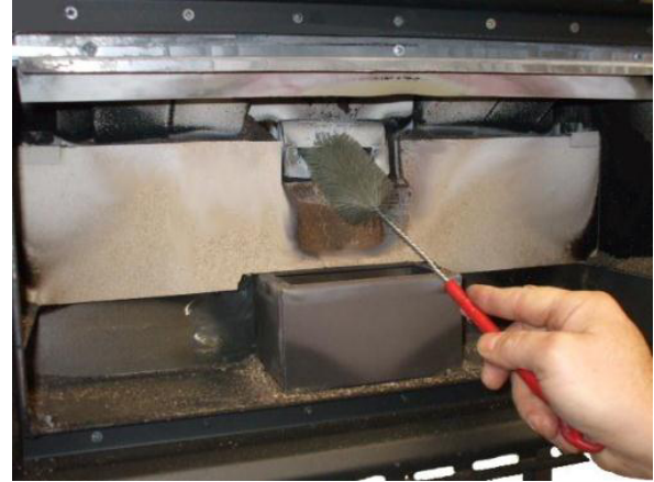
Fig. 35 - Cleaning with a brush
