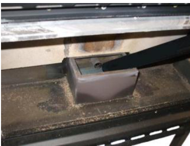
Fig. 36 - Fire pot room cleaning
