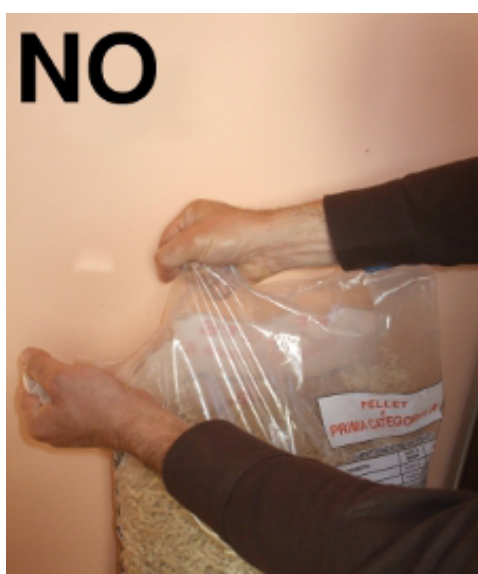
Fig. 28 - Wrong opening of the pellets bag
