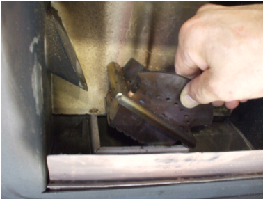
Fig. 27 - Burning pot extraction
