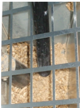
Fig. 33 - Hopper and auger cleaning
