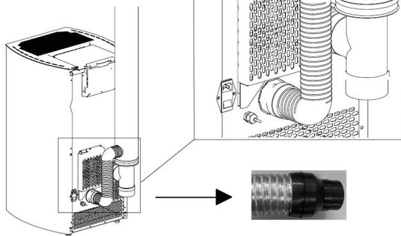
Fig. 11 - Tuyau flexible
