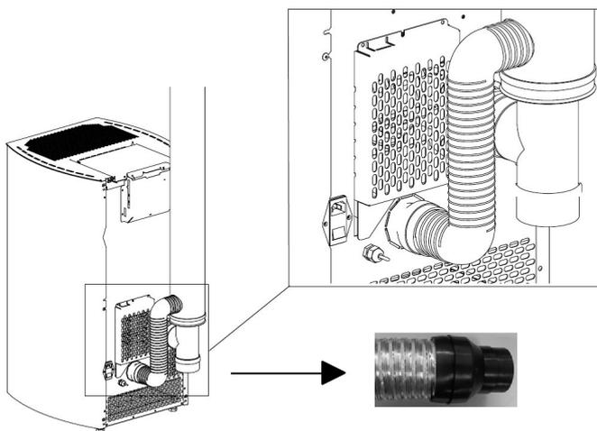
**Fig. 16 - Tuyau flexible**
